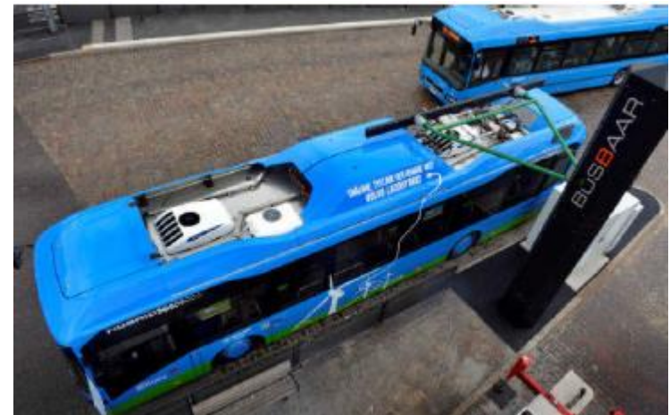
Image: Busbar system demo in Sweden
