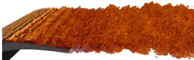
Figure 1: Snapshot of iso-surfaces of Q -criteria coloured by velocity magnitude in the wake of a single T106D low pressure turbine blade [7].
