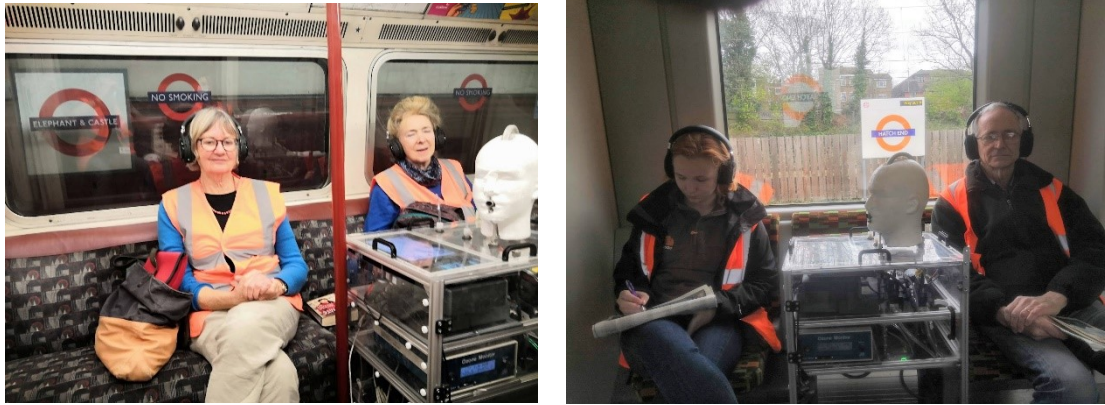
Figure 4.3: The positioning of MoRS between the participants measuring at the breathing height of the participants on a subway journey (left) and an Overground journey (right).
