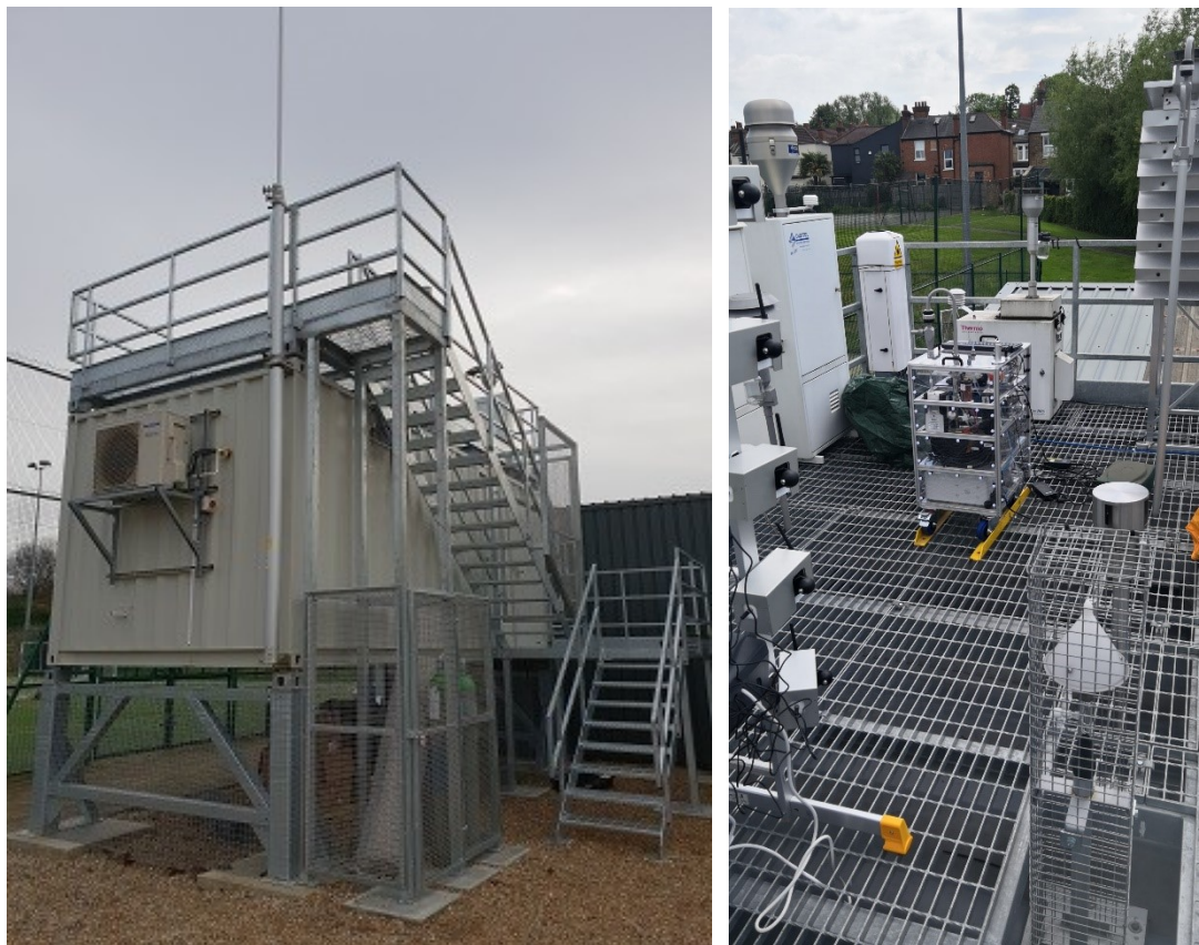
Figure 3.7: The Mobile Reference Station (MoRS) located at the Honor Oak Park, urban background site, for instrument intercomparisons and co-locations with reference instruments at the site.
