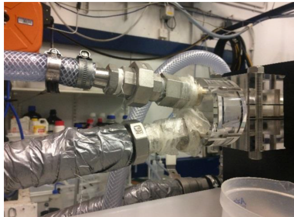
Figure 4.5: Inlet section wrapped with a plastic film to help minimise air leakage.
