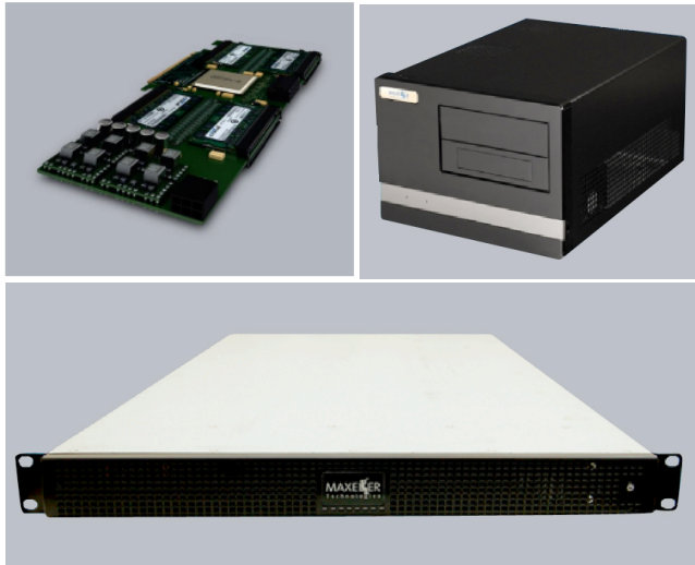
Figure 2. Sample Maxeler systems the NeuroFlow neural simulator run on. Upper left: A single system board containing one FPGA; upper right: workstation with a single FPGA card; bottom: a 1U server unit.
