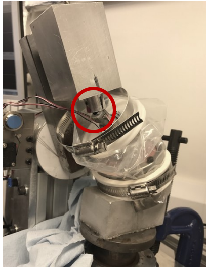
Figure 5-33 The collapsed connector
