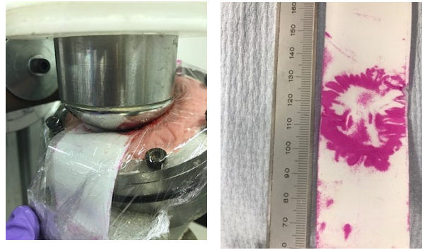
Figure 6-5 Illustrations of (a) fujifilm position between the implant and glenoid sample, and (b) the contact area measuring using Fujifilm
