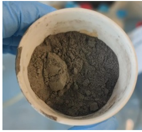
Figure 3.3 As-received coal fly ash from power plant
