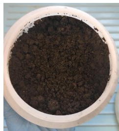
Figure 3.4 Digested sludge from sewage sludge anaerobic plant
