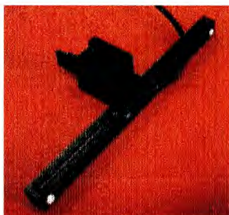
Figure 7.3: Optical tracking IRED mount for monitoring the trigger motion.
