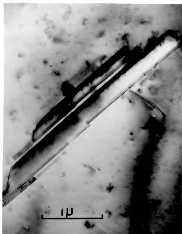
Figure 4.30 a) Electron micrograph showing defects at a subgrain boundary in specimen AP 136/7. The interface planes as determined by trace analysis are indicated along the boundary. A cross slip loop is marked L. b) A micro-twin present in a different area of the same specimen (multibeam reflection).
