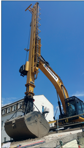
Figure 7. The innovation programme led to use of telescopic clamshell excavators on other projects following successful trials at Paddington, which found excavation rates increased from 48 m 3 /h to 54 m 3 /h
