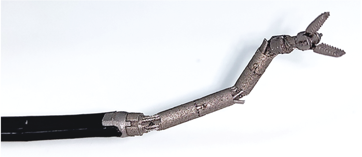
Figure 3.5: Flexible 3mm instrument prototype for snake-like robots. The instrument was 3D printed in stainless steel and uses tendons for actuation. (Source: [27]) © 2020 IEEE
