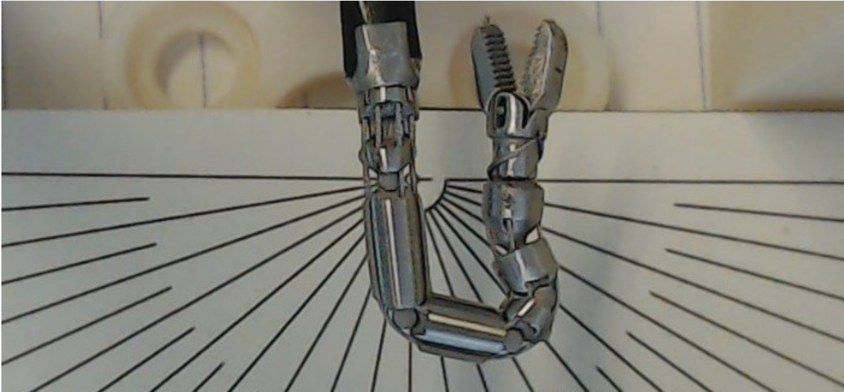
Figure 3.22: The measurement position of the instrument to determine the maximal joint angles. (Source: [26]) © 2019 IEEE
