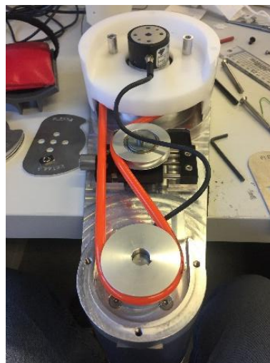
Figure 3.5. The transmission system with polyurethane belt and tensioner pulley. Tension is achieved by turning the push screws, drawing the tensioner pulley across the belt.
