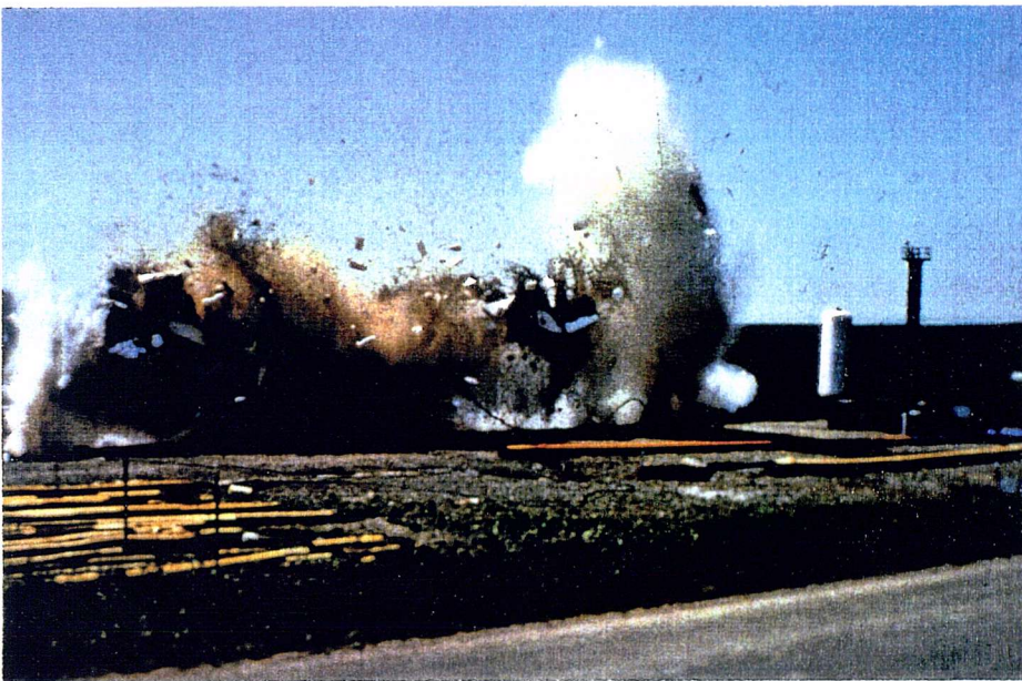
Fig. 1.1 Rapid crack propagation in a full scale test on a gas pressurised pipe
