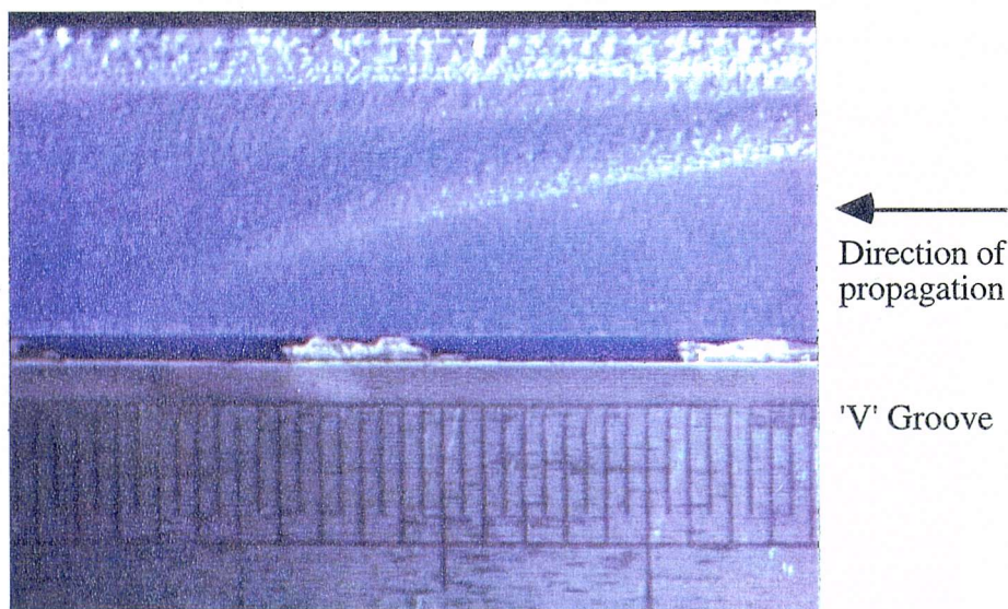
Fig 7.18 Picture of arrest line seen on specimen tested at a striker velocity of 7.5 m/s
