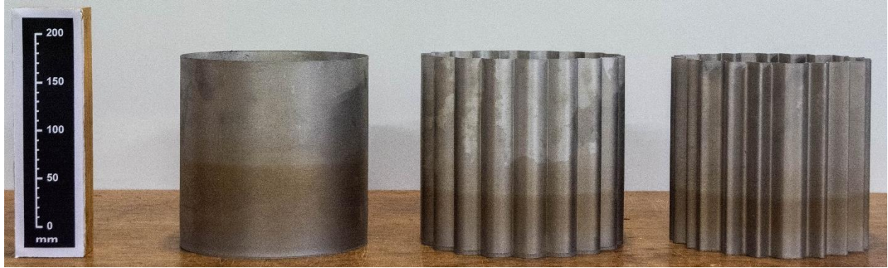
Fig. 5 Photograph of three types of PBF shell specimens (from left to right: circular, Aster and wavy)
