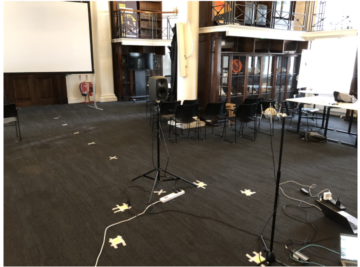
(b) SRIR measurement setup for the front position. Reproduced from Daugintis et al. 2024.
