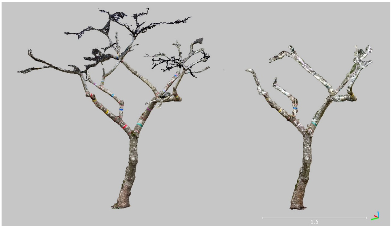
Figure 3) Point clouds of 11 cm dbh Cornus nuttallii specimen generated using (left) photogrammetry (DTP model), reconstructed from two scans each of 250 photos and (right) LiDAR (LiDAR model) and the Polycam app on an iPhone 12 Pro, placed side-by-side in CloudCompare. Scale bar shown in metres.
