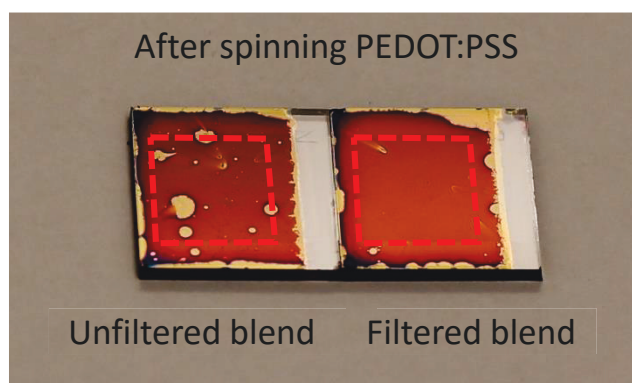
Figure 3.21: Inhomogeneity in the PEDOT:PSS layer caused by aggregates in the underlying unfiltered P3HT:PCBM blend film, compared to a more uniform PEDOT:PSS coated on a filtered P3HT:PCBM blend film (the approximate region where the 6 pixels would subsequently lie are marked out in red dashed boxes).
