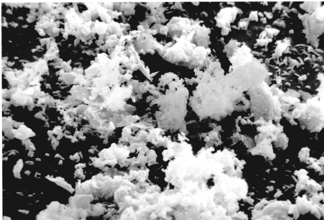
Figure 72. Electron Micrograph of Deposit formed from the Combustion of a 2:1 Blend of Coals 1 and 3, showing the presence of non-crystalline particles.
