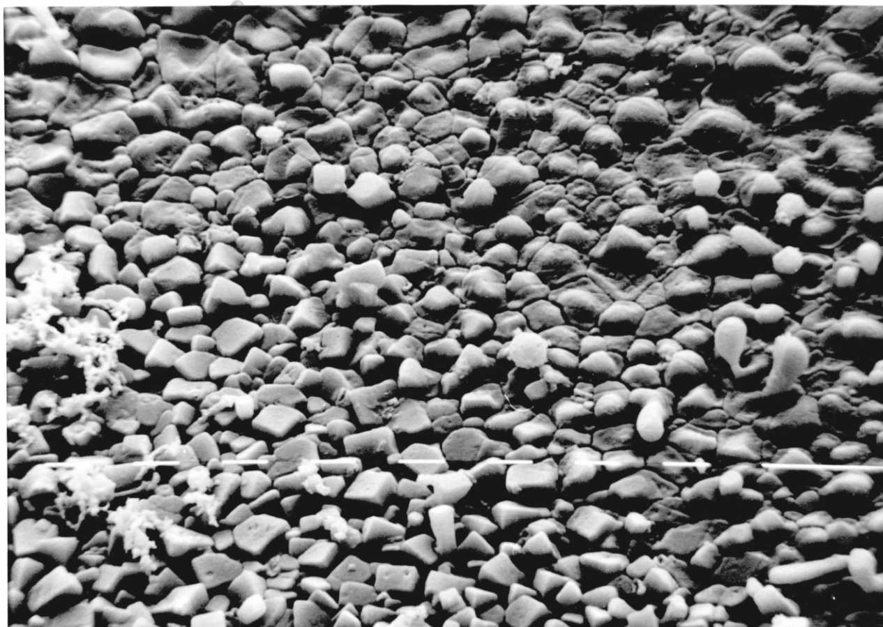
Figure 61. Electron Micrograph of Deposit from Coal 1 Combusted in a Limestone Bed, showing cubic and partially fused halide crystals.
