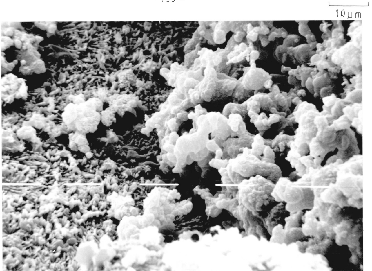
Figure 65. Electron Micrograph of Deposit from Coal 1 Combusted in a Dolomite Bed, showing deposit build-up.
