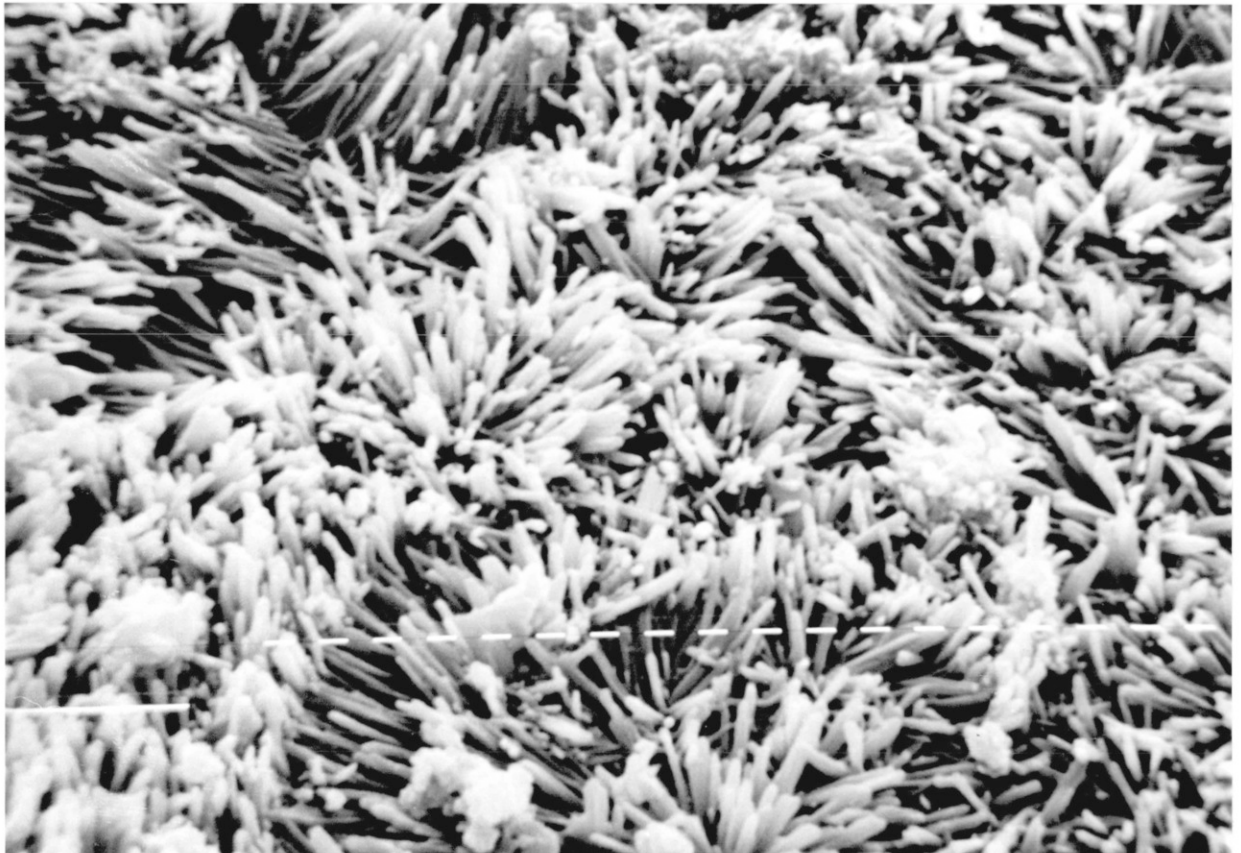
Figures 64a and b. Electron Micrographs of Deposit from Coal 1 Combusted in a Dolomite Bed, showing Calcium rich needle-like growths.
