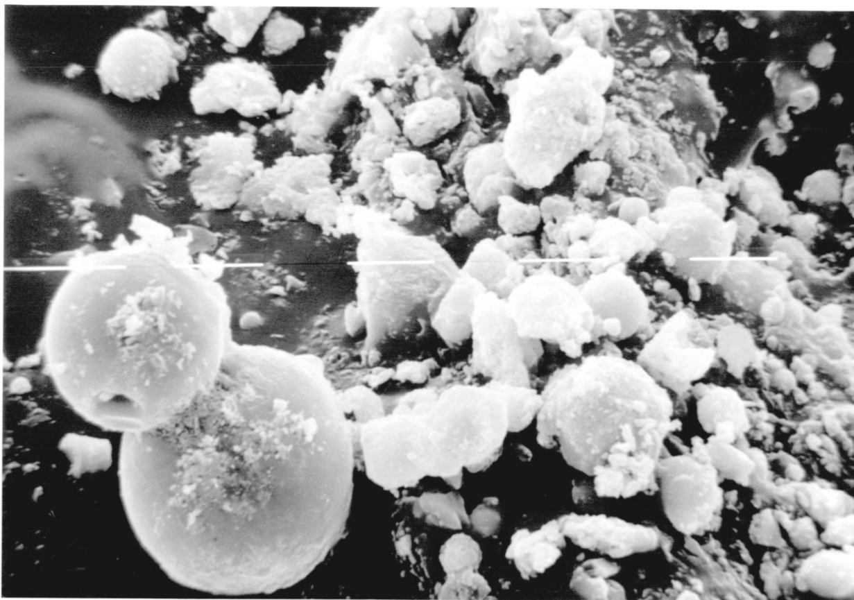
Figure 81. Electron Micrograph of Ash from Coal 1 after Bomb Combustion, showing crystalline and fused particles.
