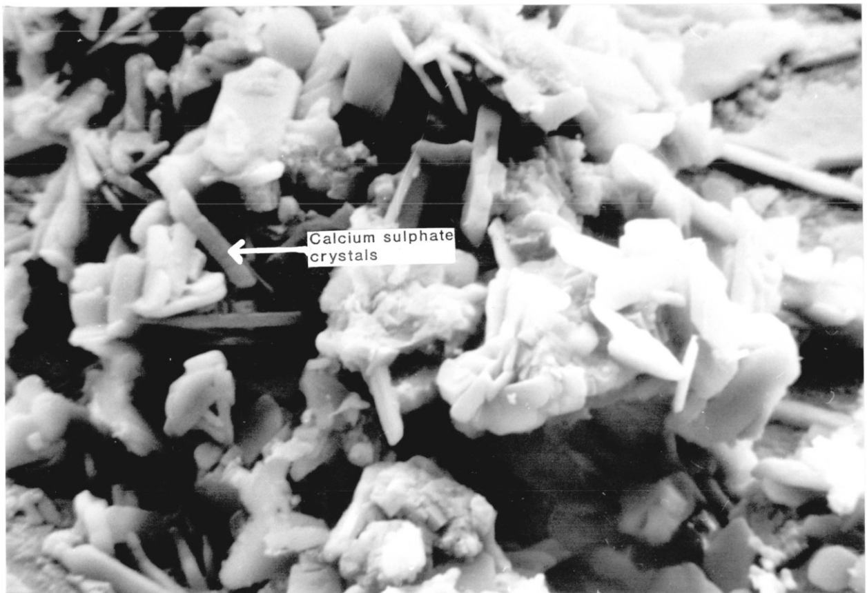
Figure 76a and b. Electron Micrographs of Deposit formed from the Combustion of Chlorine Enhanced Coal 1, showing the predominance of Calcium Sulphate crystals.
