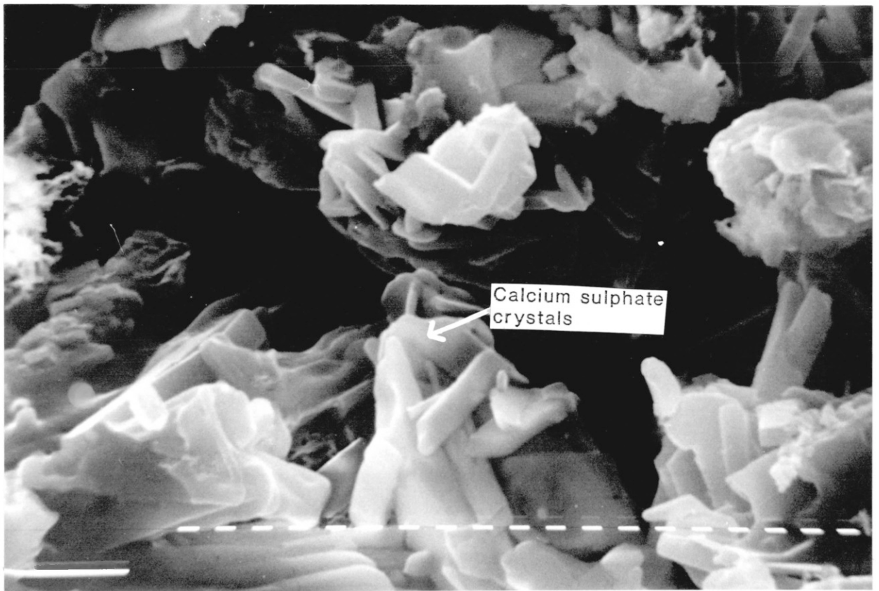
Figure 48. Electron Micrograph of Deposit from Coal 1 Combusted in a Lower Fluidising Gas Velocity (0.13 m sec -1 ) showing abundance of Calcium and Sodium Sulphate crystals.
