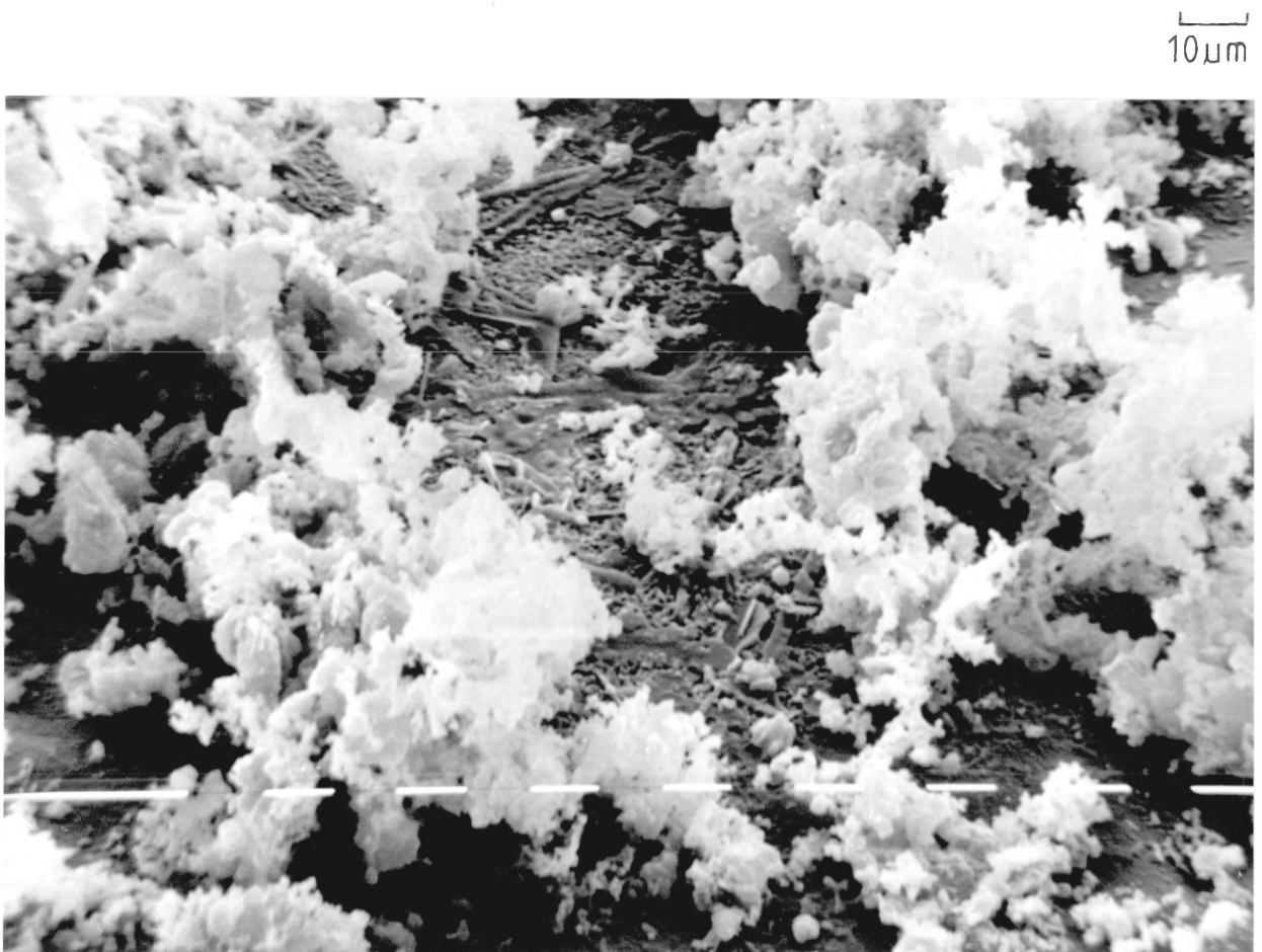
Figure 66. Electron Micrograph of Deposit from Coal 3 Combusted in a Limestone Bed.
