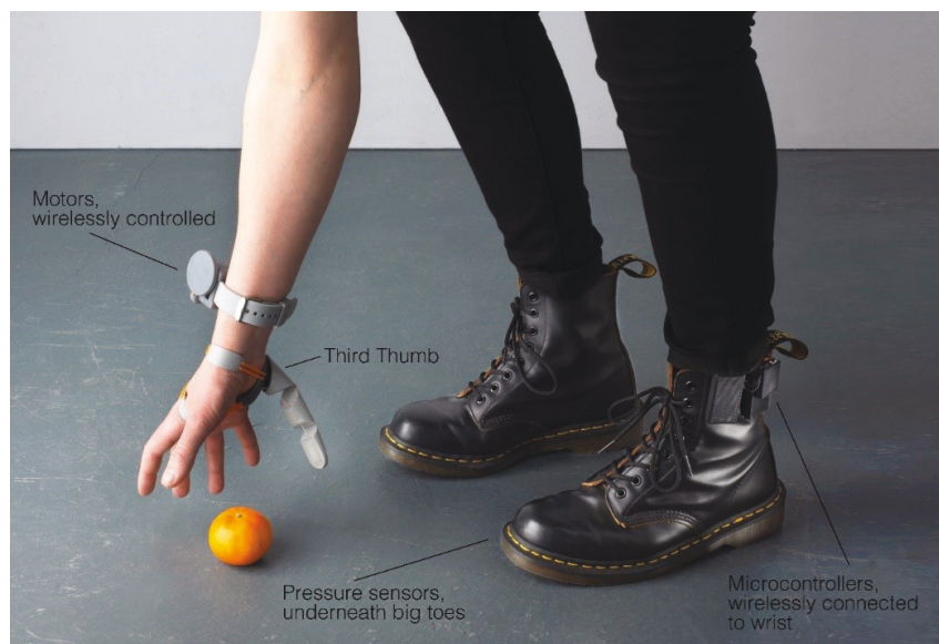
Figure 1-1: Artificial supernumerary limb model 'Third Thumb' by Dani Clode Design for enhanced dexterity. The artificial thumb is mounted to the wrist and equips the user with two sDoF. The Third Thumb is driven via
