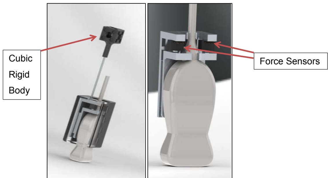
Figure 4.1 The ultrasound probe. The image on the left shows the ultrasound probe inside a plastic casing with a cubic rigid body that housed the 12 infrared optical markers. The force sensors are highlighted in the image on the right. (8) .
