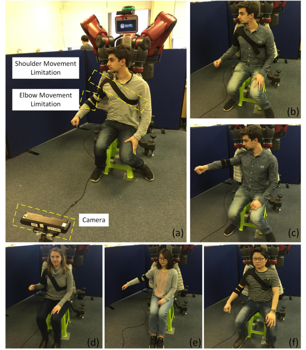
Fig. 2: The experiment environment set up. Four different healthy users (ages 23-32, mean:28, std:2.19) wear braces to simulate 6 scenarios including elbow, shoulder, and elbow-shoulder movement limitations.
