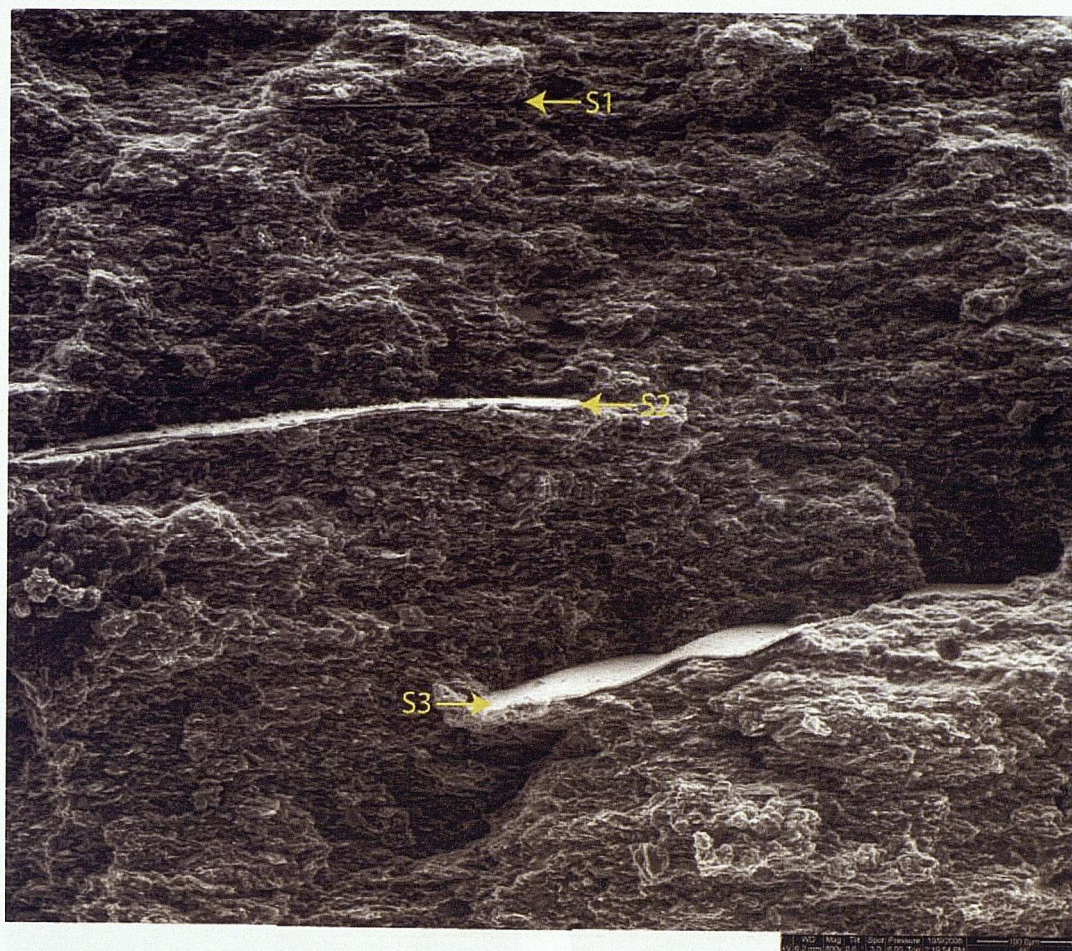
Figure 10.3 Montage of a grid of sixteen SEM images taken of the surface of the Oxford Clay. S1, S2 and S3 = shells. Scale bar bottom right image, approximately 1.2mm across image.
