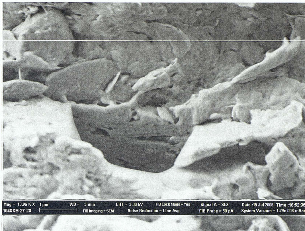
Figure C.13 Focussed ion beam image of the Oxford Clay, showing clay particles with clay mineral cement between particles.
