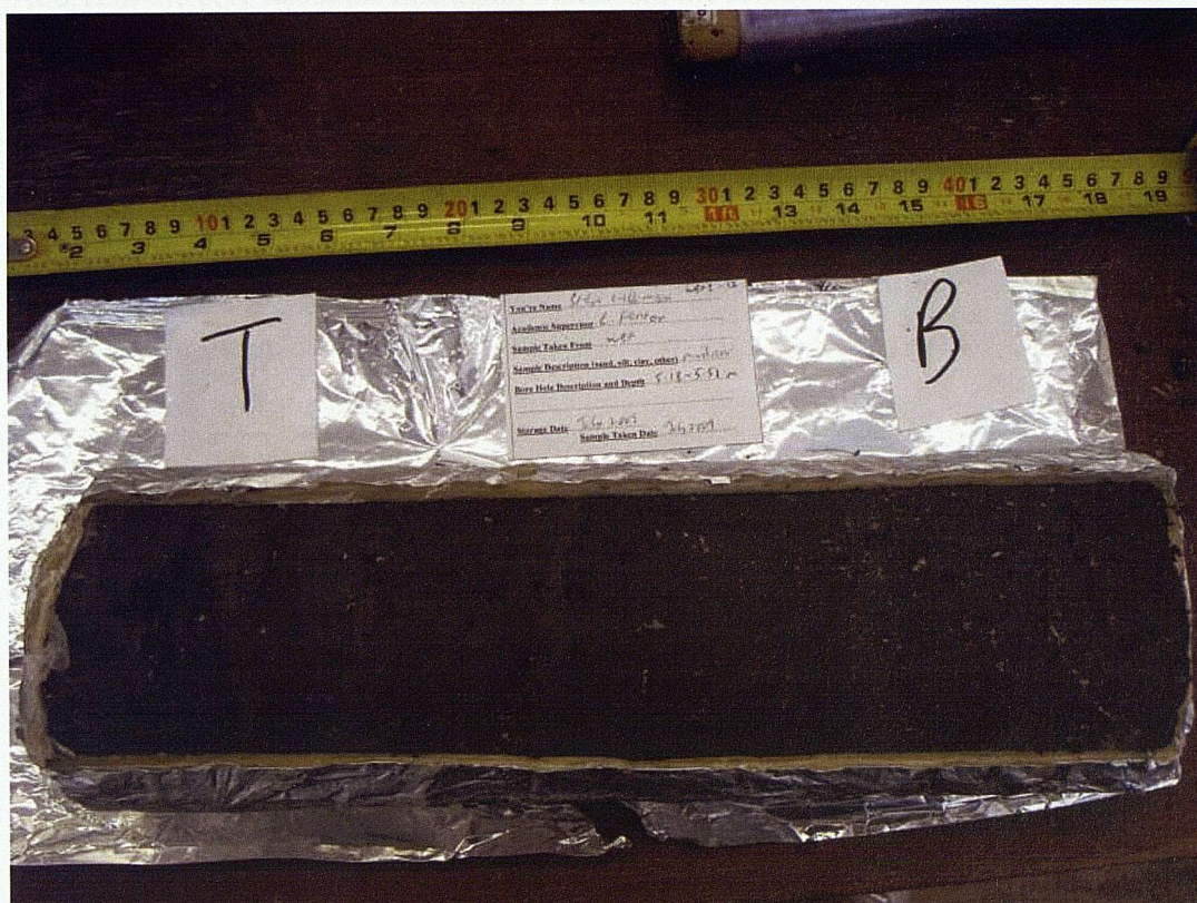
Figure 7.12 Kimmeridge Clay, core WBF1, 5.18-5.51m mudrock becomes coarser grained, and contains some shell fragments. T = top of core B = base of core, tape measure showing cm (top) inches (bottom).
