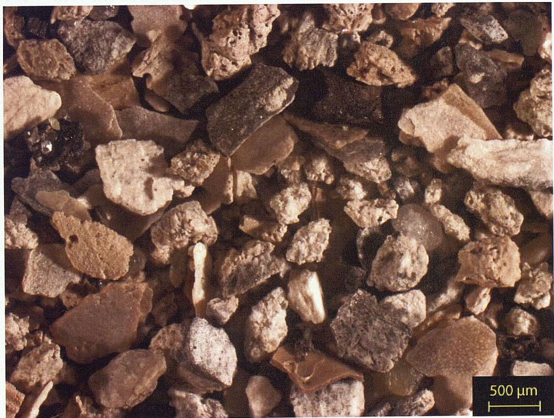
Figure 7.18 The greater than 160 micron fraction residue of the 12.71m sample, the residue is rich in polyminerale lithic fragments. There are a few broken shell fragments, and very few quartz grains.
