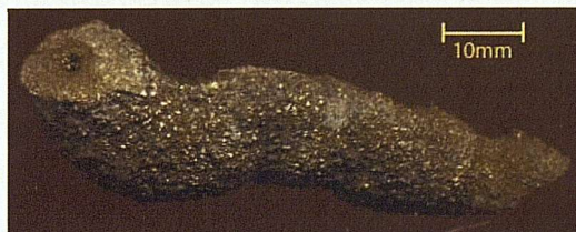
Figure 6.7 Pyrite nodules from the Gault Clay at Barrington.
