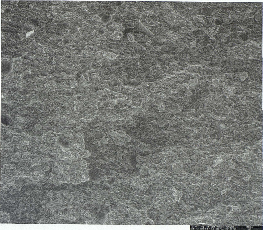
Figure 10.8 Montage of 16 images of a vertical broken surface taken from a block sample of Gault Clay. This samples shows a preferred particle orientation. It shows the particle orientations in an area which has not been altered by the presence of joints.
