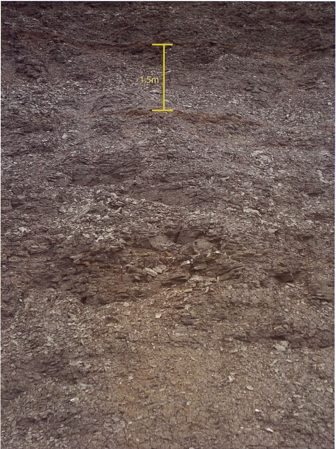
Figure 5.14 The quarry face at Stewartby, the red bands in the image probably mark pyrite rich layers within the Oxford Clay. There are also other shell/concretion rich bands which cannot be picked out in this image. Image taken facing south west.
