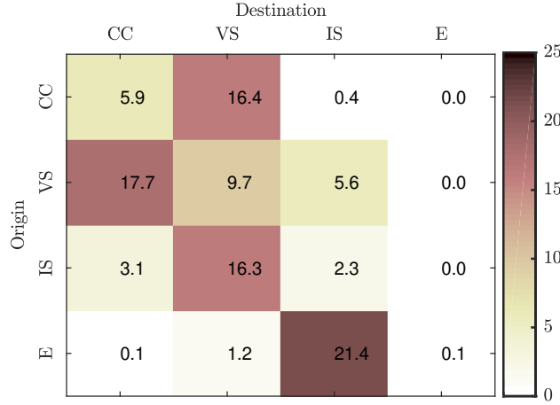
Figure 5.4: Origin-destination matrix for particle final locations according to zones. Figure shows the percentage wise distribution of particles based on the zone of origin at the time of seeding and the zone where they end up at time t^* = 0.67 .
