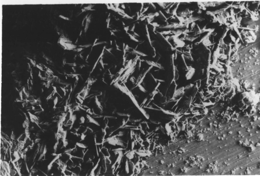
MA956 ( \text{Fe}_{20}\text{Cr}_{5}\text{Al} ), preoxidised 20 min. at 1100^{\circ}\text{C} in air, 90h, high p\text{S}_2 , 1123K. Damage near to suspension hole X100
