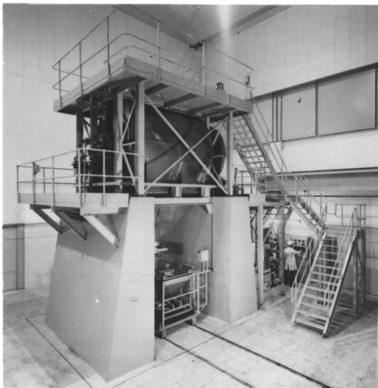
High energy ball mill used to produce mechanical alloys at the Wednesbury plant
