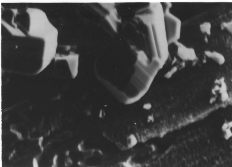
Alloy D ( \text{Fe}_{25}\text{Cr}_{6.5}\text{Al} ) preoxidised 1h at 1100^{\circ}\text{C} in air, 204h, high p\text{S}_2 , 1123K X2k
