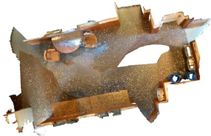
Figure 6. An example of a point cloud for the interior of a building.
