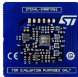
Figure 4-10 Schematic of STMicroelectronics STEVAL-SMARTAG1 with the overall dimensions of 43 × 43 mm.
