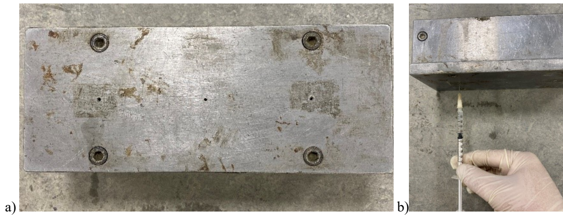
Figure 6-2 Customized 50 × 50 × 50mm steel mould with a) 2mm diameter drilled holes and b) 1ml syringe with the needle inserted at the bottom of the base plate.
