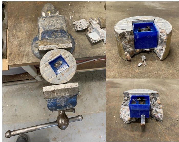
Figure 5-2 Retrieving RFID MEMS sensors from concrete samples after 7 months of embedment.
