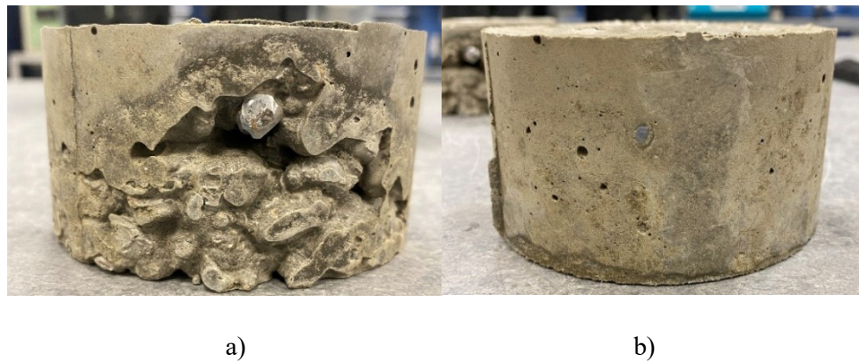
Figure 4-41 High strength concrete 14 days cured specimens with a) improper and b) proper compaction.
