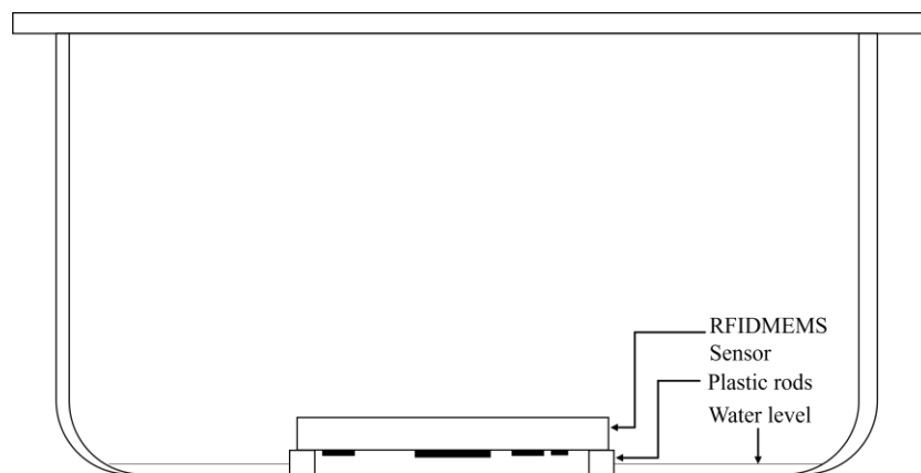
Figure 4-36 Directly exposing RFID MEMS sensors to 100% RH humidity.
