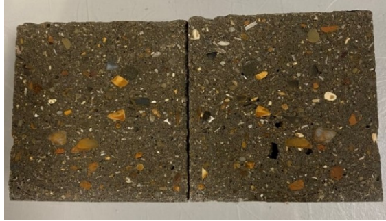
Figure 6-8 Cross-section view of 50% aggregate volume mortar sample with 0.6 ml of injected air after 1 minute of vibration.
