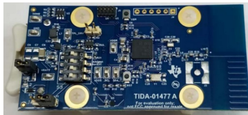
Figure 4-6 Schematics of Texas TIDA-01477 Humidity and Temperature Sensor Node with the overall dimensions of 76.2 × 38.1 mm and HDC2010 humidity sensor attached.
