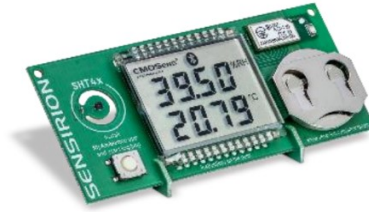
Figure 4-8 Schematics of Sensirion Smart Gadget with the overall dimensions of 75 \times 32 mm and SHT4x humidity sensor attached.
