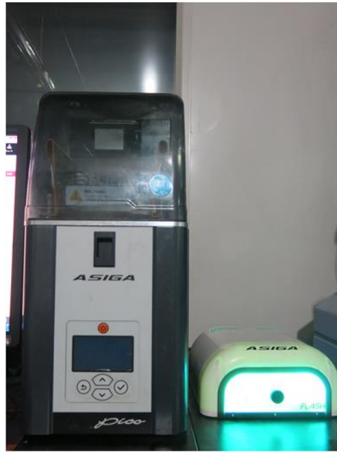
Supplementary Figure 4 | Optical image of the 3D printer (FREEFORM PICO 27, AISGA, USA) adopted in this study for generating the anisotropic polymer architectures.
