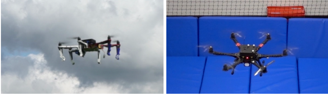
(a) Tracking and landing on a moving target. (b) Fault detection and recovery despite the loss of an actuator. Two cameras were used for localisation and target detection. [Tzoumanikas et al., 2019] MAV maintains control of position and yaw. [Tzoumanikas et al., 2020b]
