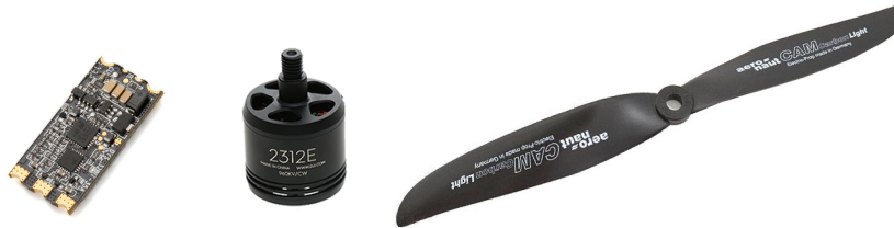
(b) Propulsion system #2 consists of the bidirectional capable DYS 35A Aria ESC, the DJI 2312E 960Kv motors and the carbon reinforced Aero-naut CAMcarbon Light 9545 propellers. In order to cope with the large angular acceleration/deceleration due to direction change, the propellers were secured with elastic stop nuts.
