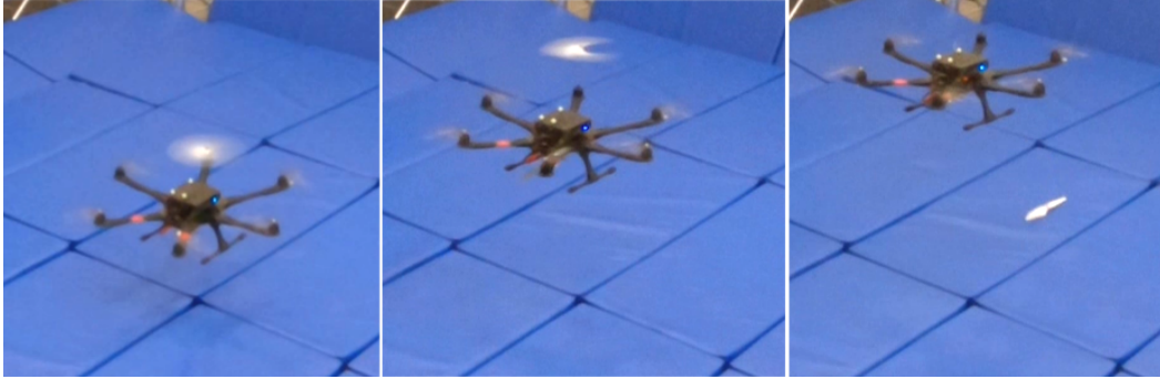
Figure 4.1: Our MAV experiencing a propeller loss. The fault is identified online, the failsafe enabled and the MAV can still control its position and orientation.
