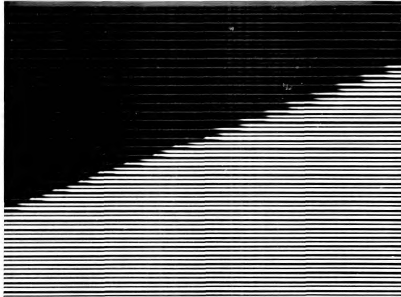
FIG. 5.13 Contour and Linear Interpolation. Signal Distributor Aperiodic; Interlaced Fields at 50 C.P.S. Horizontal Bandwidth, 20^\circ Contour, Magnification X7; Bromide WSG 3S.
