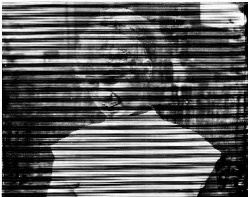
FIG. 5.16 Single Field. 200 Lines, Horizontal Bandwidth 100 C.P.S; Bromide WSG 4S.
