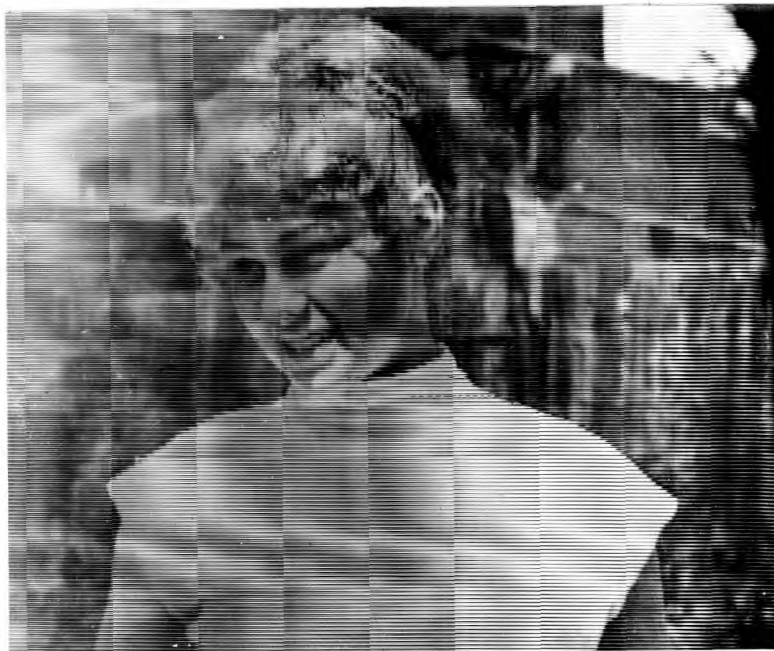
FIG. 5.20 Contour Interpolation . 400 Lines at 50 C.P.S. Horizontal Bandwidth; Bromide WSG 4S.
