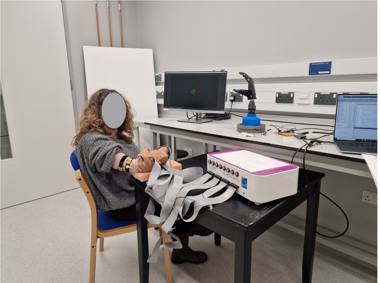
Figure 4.8: Experimental Setup for offline validation of EMG-RS. High Density electrodes on the participant’s arm are connected to the Quattrocento amplifier. The EMG signals are sent to the laptop where they are processed and used to control a cursor on the screen, as well as the TASKA hand, which is shown here supported on the table.
