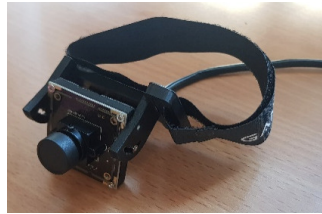
(b) Webcam is attached to an adjustable Velcro strap
