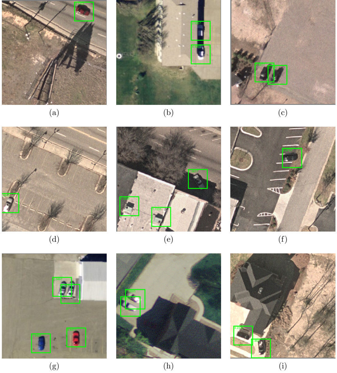
Figure 5.6: Sample regions of the test images of the OIRDS dataset after applying the ACD framework. Bounding boxes represent detections and the number at the top left corner of each bounding box represents its confidence score. Shown images are scaled for viewing.
