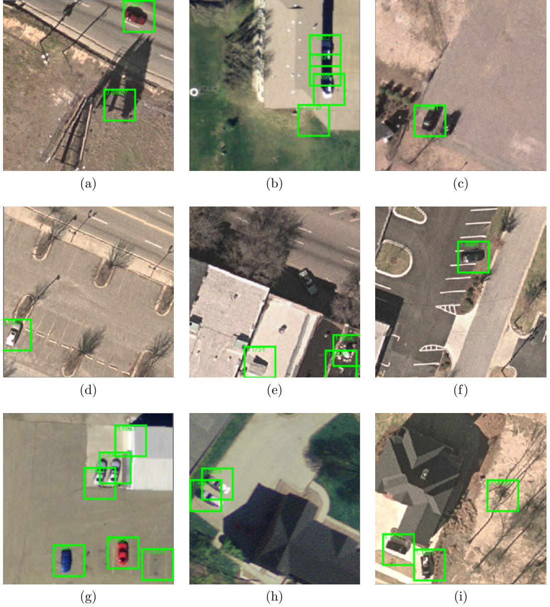
Figure 4.9: Sample regions of the test images of the OIRDS dataset after applying the proposed FCD framework. Bounding boxes represent detections and the number at the top left corner of each bounding box represents its confidence score. Shown images were scaled for viewing.
