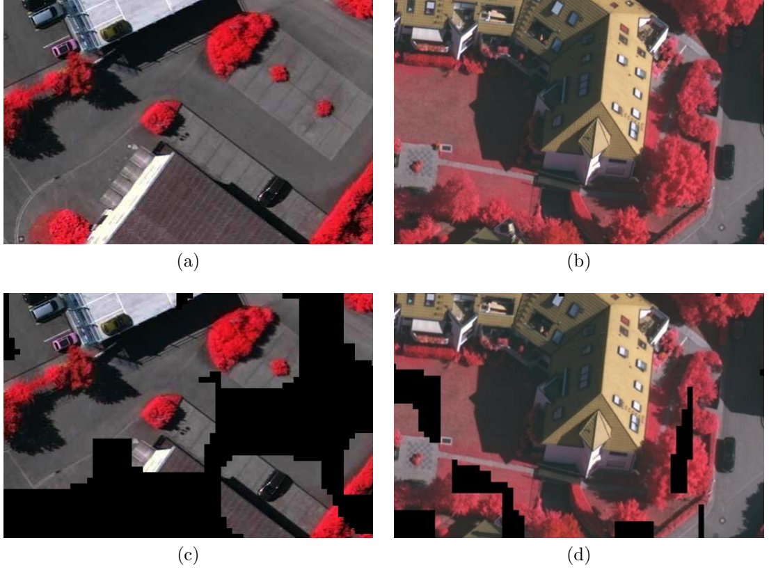
Figure 4.4: Application of the window-evaluation stage on a sample region of the training dataset: (a) and (b) original images; (c) and (d) corresponding processed images. Areas that have been eliminated by the window-evaluation stage as they are highly unlikely to contain cars are marked with black. Shown images were scaled for viewing.
