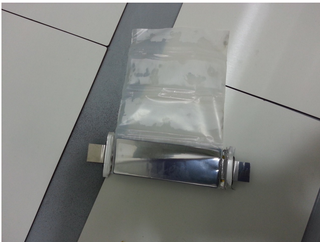
Figure 27 – Cell with pouch material removed
