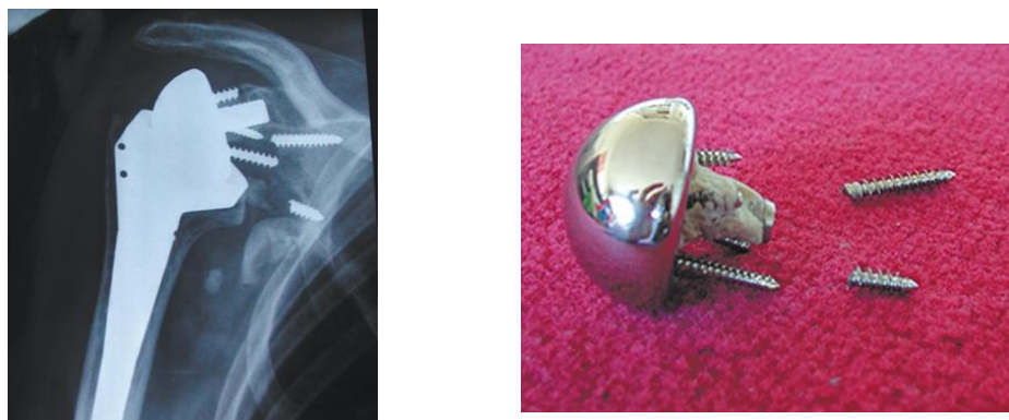
Figure 3-25 Breakage of screws in the RSA (adapted from Juvenspan et al. 2005).
