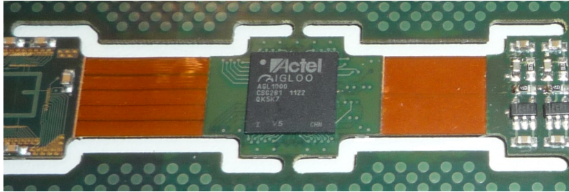
Figure 4.1: Photograph of the HMRM FPGA mounted on the monitor central PCB section. The FPGA package measures 10 mm by 10 mm by 1.05 mm.
