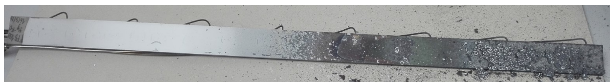
Figure 5.34 Stainless steel bar painted with FFB® 1210 paint and heat treated from 200 °C (left, cold extreme) to 1,100 °C (right, hot extreme). Detachment of paint layer was observed for temperatures above 800 °C.
