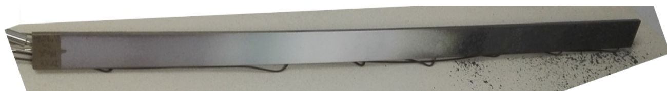
Figure 5.35 Stainless steel bar painted with IPXX phosphate binder paint and heat treated from 200 °C (left, cold extreme) to 1,100 °C (right, hot extreme). Detachment of paint layer was observed at high temperatures above 900 °C.
