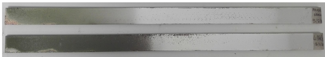
Figure 5.32 Stainless steel bars painted with lithium poly-silicate (top bar), and LithiSil®25 lithium silicate. Both bars were heat treated from 200 °C (right, cold end) to 1,100 °C (left, hot end).
