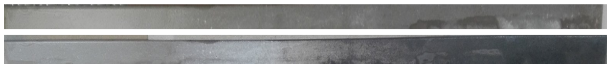
Figure 5.37 Stainless steel bar painted with Durazane® 1800, polysilazane polymer paint, shown before heat treatment (top) and after heat treatment (bottom) from 200 °C (left, cold end) to 1,100 °C (right, hot end).
