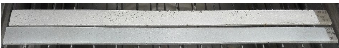
Figure 5.55 THP applied on a stainless-steel bar coated with a Ludox® SM30 interlayer (top) and THP applied directly on a stainless-steel bar (bottom), after heat treatment at 150 °C for one hour.
