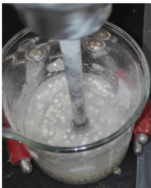
Figure 5.23 (a) Photograph of polymerized potassium silicate binder modified by lithium addition, introducing one equivalent of lithium per silica equivalent, as received by the author. (b) Photograph of lithium enriched potassium silicate binder, after water and pigment addition. An overhead stirrer was used, as well as zirconia beads to facilitate the mixing.
