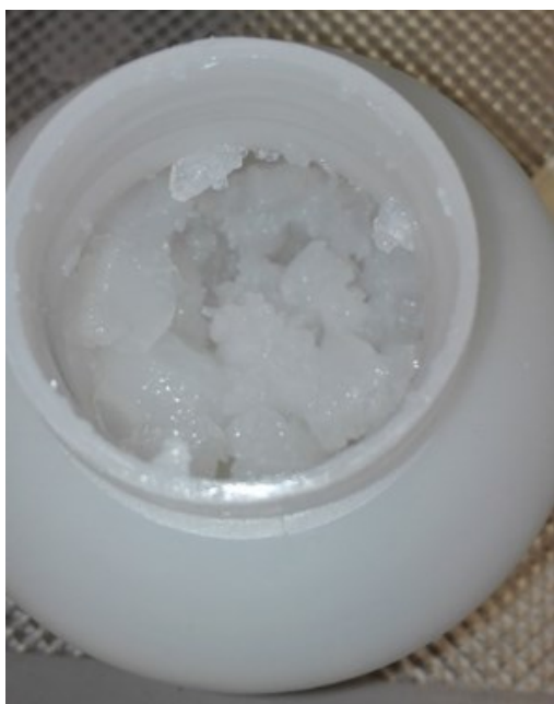
Figure 5.23 (a) Photograph of polymerized potassium silicate binder modified by lithium addition, introducing one equivalent of lithium per silica equivalent, as received by the author. (b) Photograph of lithium enriched potassium silicate binder, after water and pigment addition. An overhead stirrer was used, as well as zirconia beads to facilitate the mixing.
