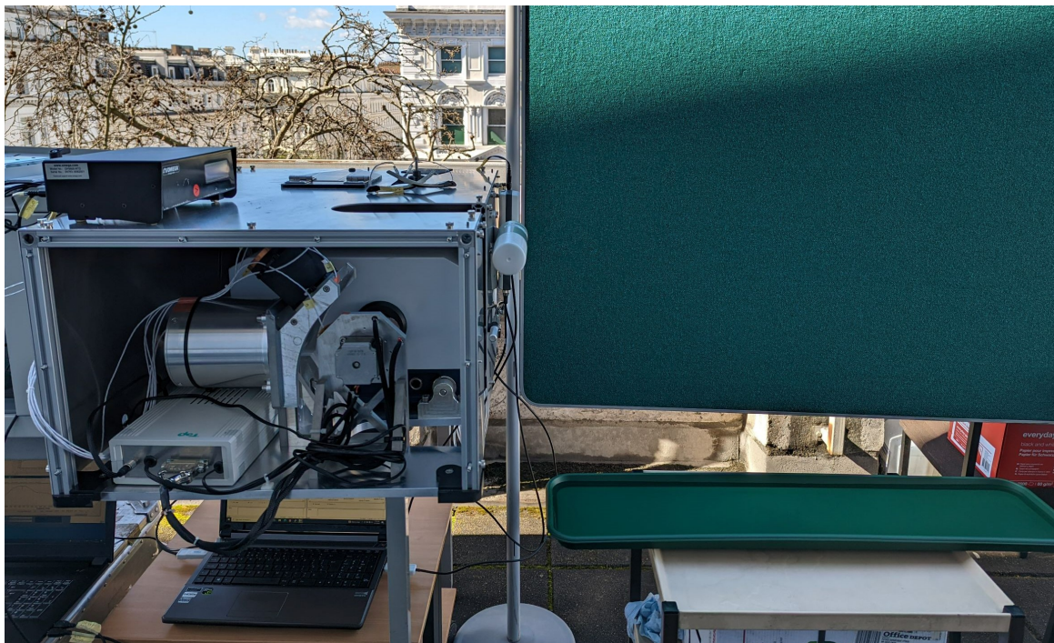
Figure 6.2: Photograph of the setup for FINESSSE to make measurements of water emissivity at different angles.
