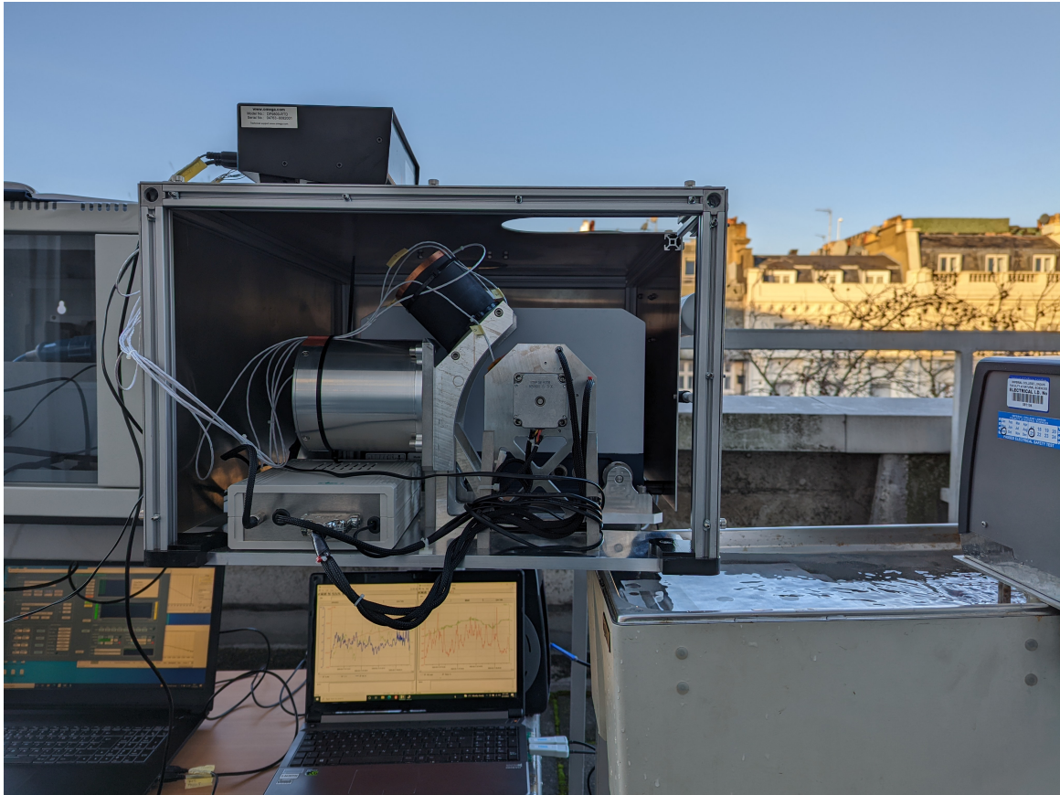
Figure 6.1: FINESSE undertaking measurements of heated water during the 3 rd set of emissivity measurements.
