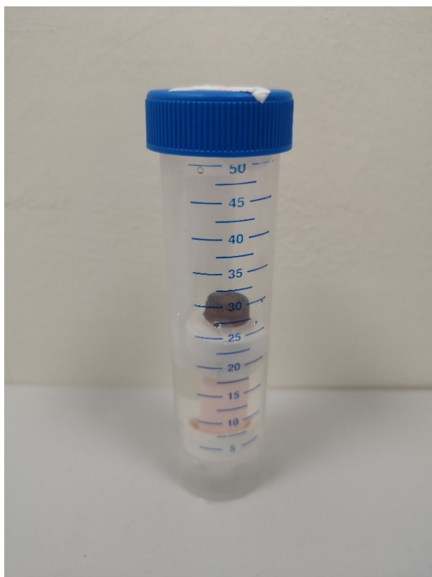
Figure 3.1 The photograph of self-assembly dialysis unit consisting of a Spectrum™ Spectra/Por™ Float-A-lyzer™ G2 dialysis device and a 50 ml plastic centrifugal tube
