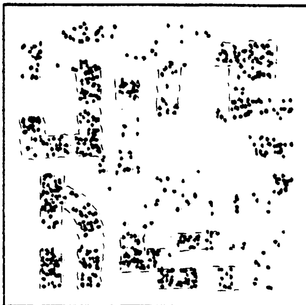
Plot E1 Magnetometer results Grid A High-pass 4 element square residual filter, radius 1 Range: \bar{x} to \bar{x} + 2\sigma Log plot Scale 1 : 200
