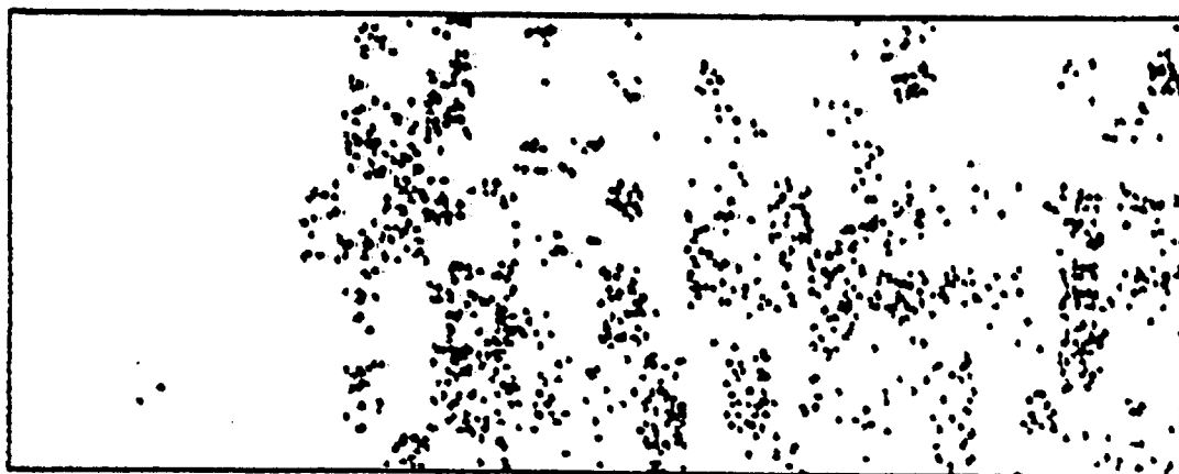
Plot A2 Dipole Dipole results Grid 1 Unfiltered data Range: \bar{x} - 0.25\sigma to \bar{x} - 2\sigma Log plot
