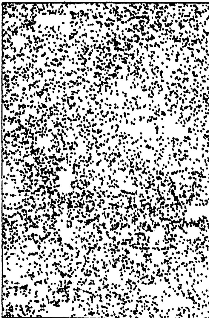
Plot 1A Dipole Dipole results Area A Unfiltered data Range: \bar{x} - 2\sigma to \bar{x} + 2\sigma Lin plot Scale 1 : 200
