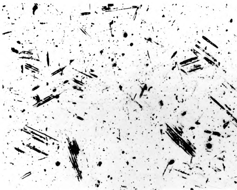
a.) Steel 347 fully softened x300
