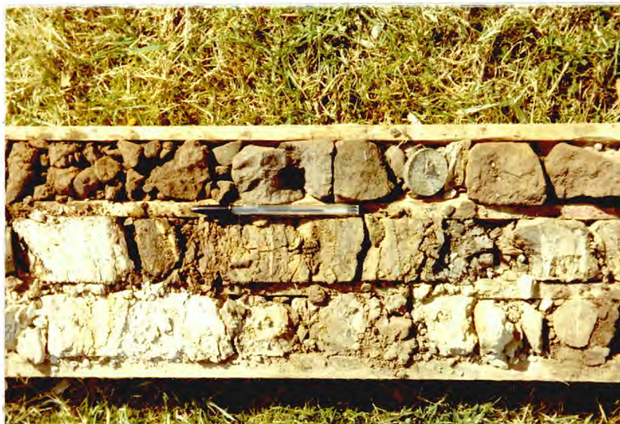
Plate 4 Drillhole K100 (69-87 ft.). Highly leached rock. Note remnant bedding planes. Scale 1:6
