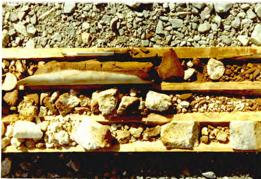
Plate 6 Drillhole K120 (156-171 ft.). Contact between unweathered rock and highly oxidized, leached material. Baryte fragments. Scale 1:6
