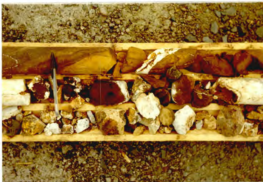
Plate 5 Drillhole K120 (144-156 ft.). Partially to moderately oxidized and leached rock. Baryte veins. Scale 1:6
