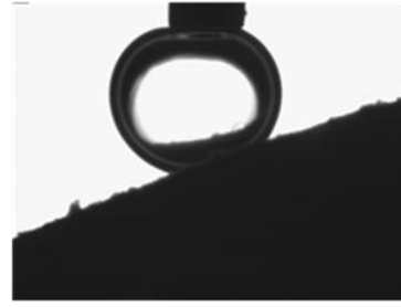
Figure 2.15: A drop of CO 2 generated from a capillary tube is brought into contact with a porous plate substrate angled at 21°. The bulk phase is de-ionized water ( P = 48.9 MPa).
