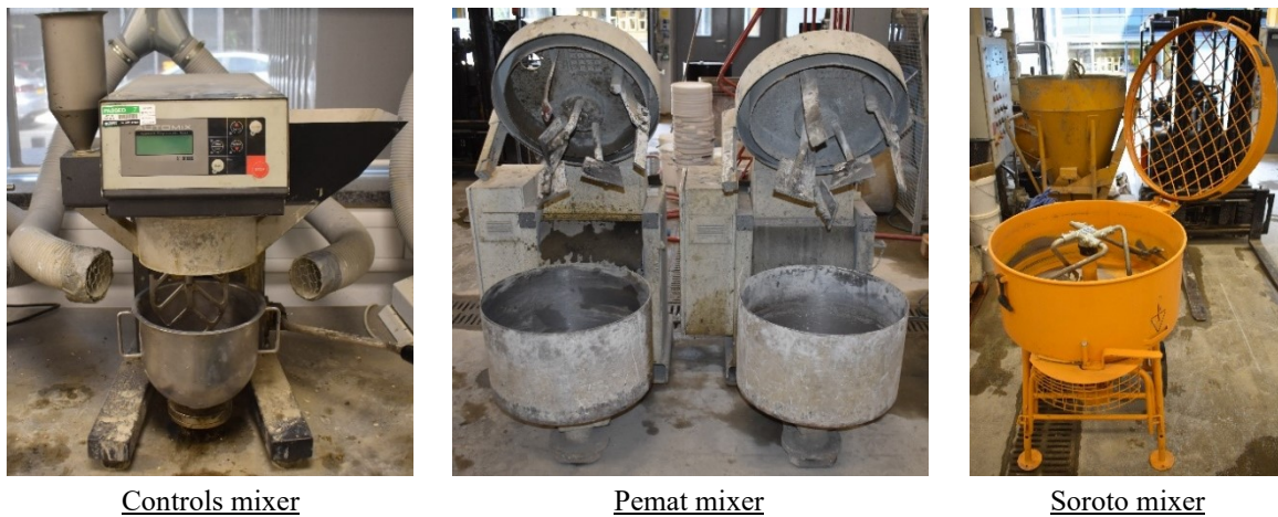
Figure 3.13 – Mixers used to prepare developed UHPC mixture
