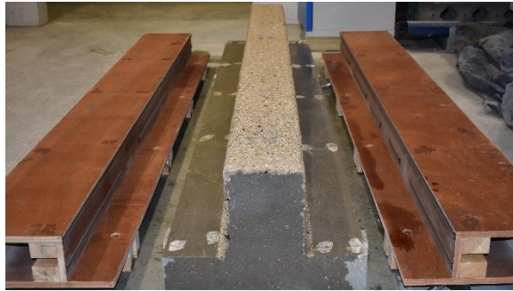
Pre-wetting of RC beam
