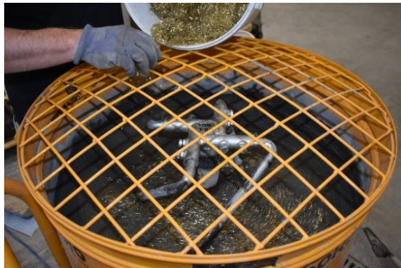
Phase 5: Gradual addition of fibres
