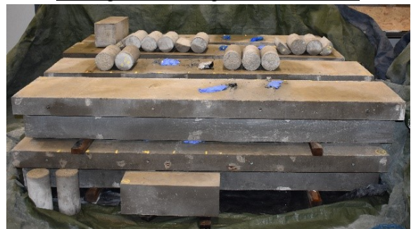
Moist curing of all beams and control specimens
