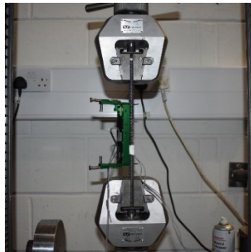
Test setup and instrumentation – \phi 10 bar
