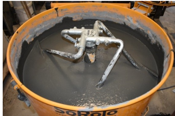
Phase 4: Wet mixing (Final)
