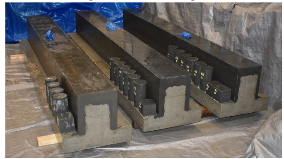
Curing of jackets and control specimens of group 2
