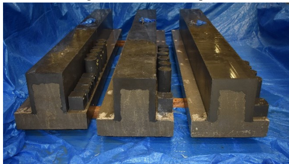
Curing of jackets and control specimens of group 1
