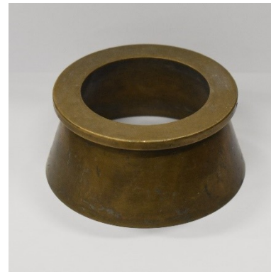
ASTM C230/230M cone (ASTM, 2014)
