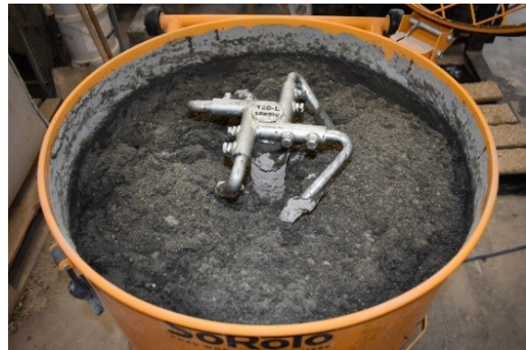
Phase 2: Wet mixing (Initial)
