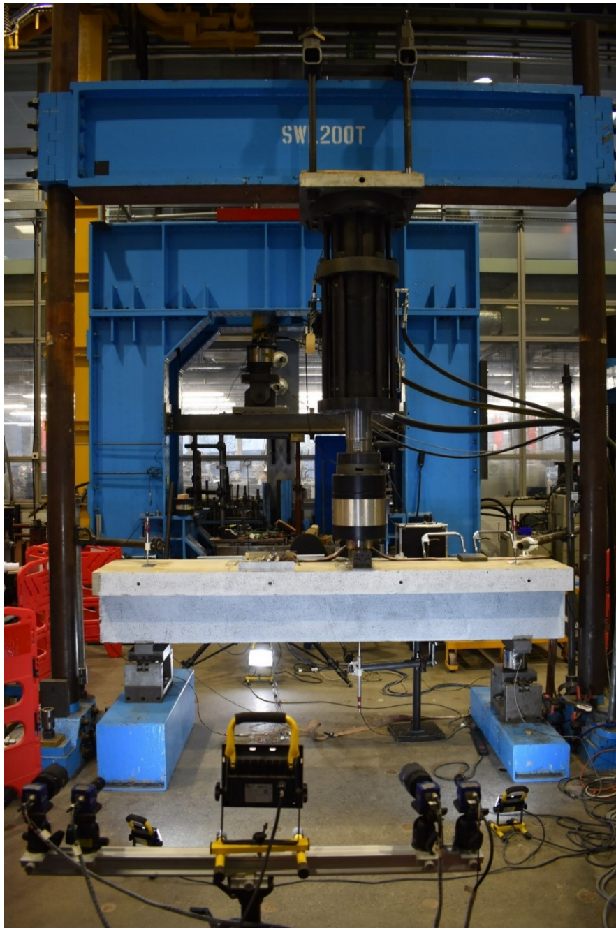
Figure 3.31 – Typical experimental set up of beam specimens
