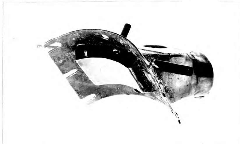
Cooling Water sampling scoop
