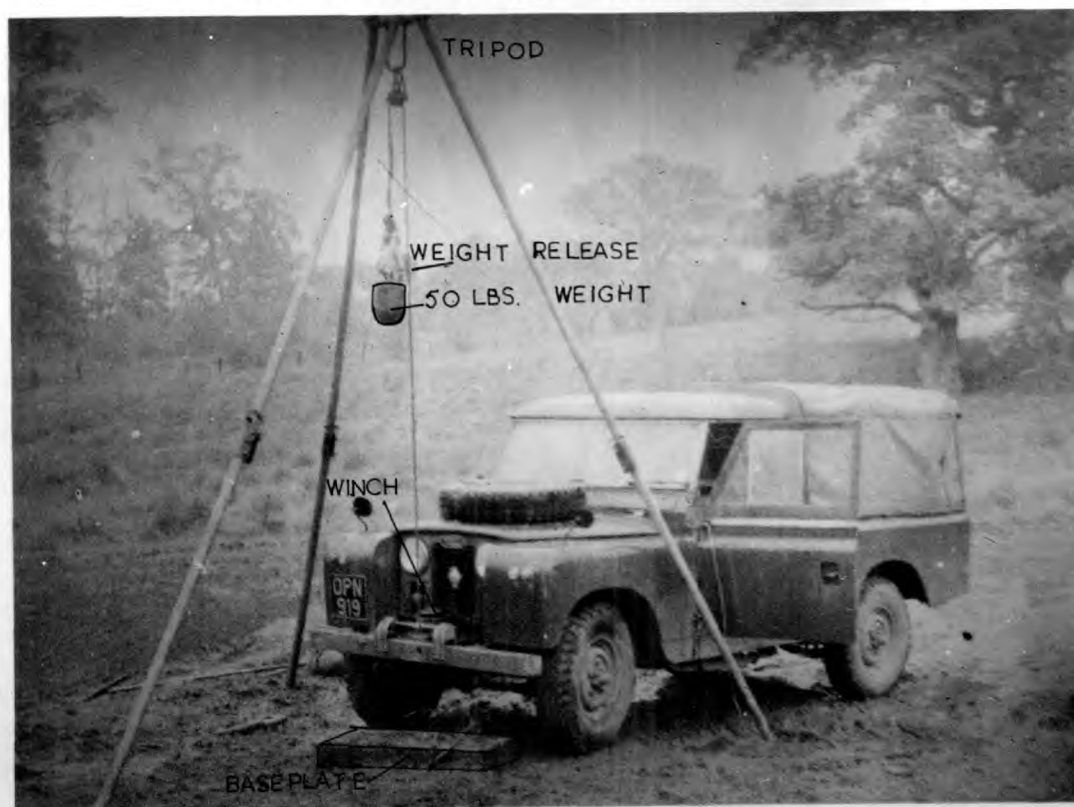
FIG 7 — WEIGHT DROPPING SOURCE
