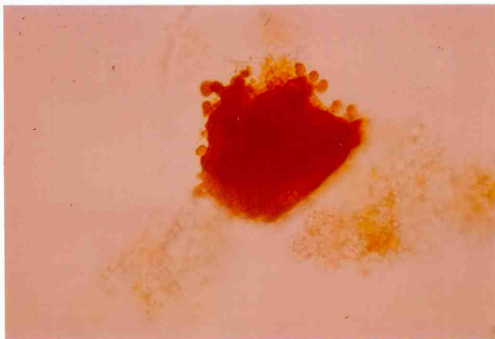
Plate 23. Photomicrograph of sediment sample CATO 10, showing orange shards of volcanic glass. 360 X.
