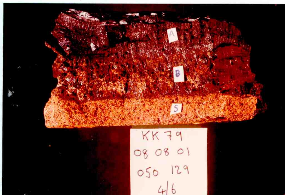
Plate 2. Sample O50 4/6. Phillipsite substrate (Zone S), showing probable replacement by Fe-Mn oxide (Zone B). The crust exhibits laminations on a millimetre scale, and has a smooth upper surface. Scale as in Plate 1.
