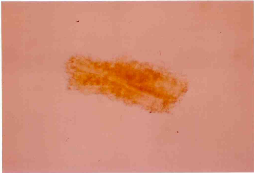
Plate 18. Photomicrograph of sample K2-1, showing a development of a phillipsite twin through the replacement of volcanic glass(?). 720 X.
