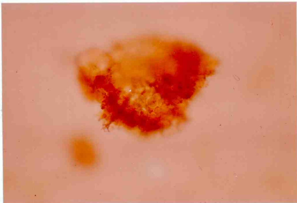
Plate 7. Photomicrograph of sediment sample K3-2, showing closely associated Fe oxyhydroxides, clay minerals and biogenic silica. 720 X.
