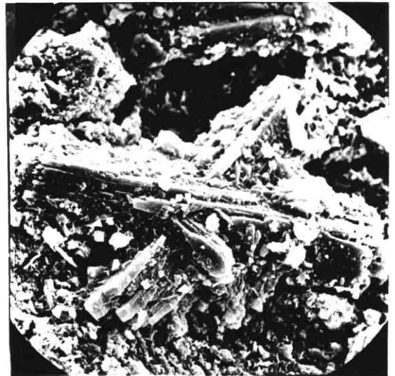
Plate 20 K2-11. Etched phillipsite twin. 1100X.
