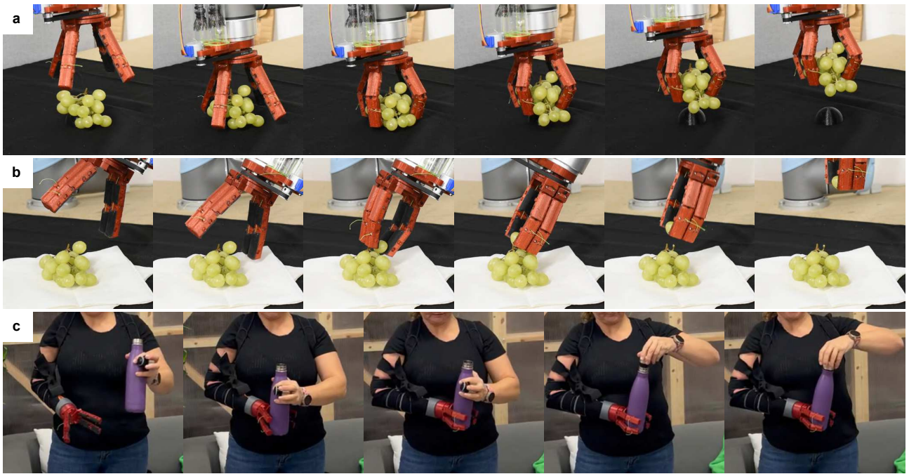
Figure 5.14: A demonstration of the Hydra Hand on a challenging manipulation task and in use as a prosthetic hand. a Using spherical mode to grasp a bunch of grapes via caging. b Using precision mode to pick a single grape from the bunch. c The Hydra Prosthetic Hand being used to grasp a bottle of water by an end user.
