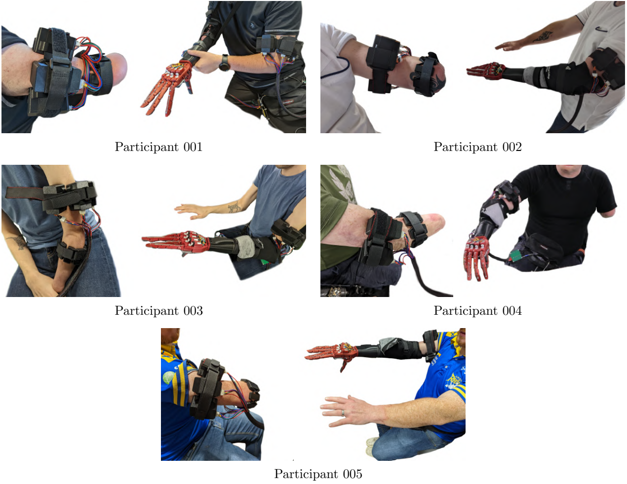
Figure A.1: Experimental setup for each participant with limb difference. Experimental setup for each participant with limb difference for stages 1 and 2 (left), and 3 (right). During stages 1 and 2, participants wore only the electrode armband and haptic feedback armband, while the prosthetic hand was desk-mounted. During stage 3, participants also donned the prosthetic hand. Note that participant 001 used an elastic sling to support the prosthesis due to having a short residual limb, and wore the haptic feedback armband on the opposing arm during stage 3 due to space constraints.
