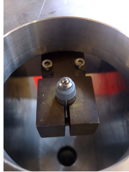
Fig. 31 Set up for R-curve measurement with the LVDT.
