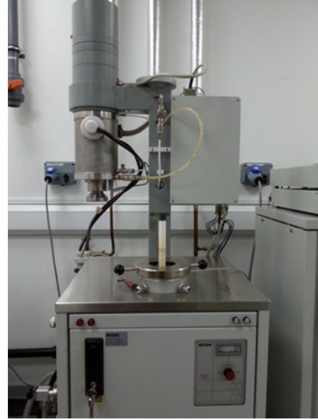
Fig. 33 Laser flash analysis employed to analyse the thermal diffusivity of tested samples.
