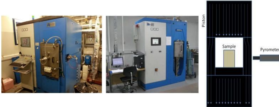
Fig. 21 On the left the graphite furnace used at Imperial College London and on the right the SPS employed at Queen Mary College. A schematic representation of the graphite crucible employed in the SPS is reported.
