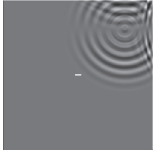
(b) Cracked plate at t = 25 \mu\text{s}
