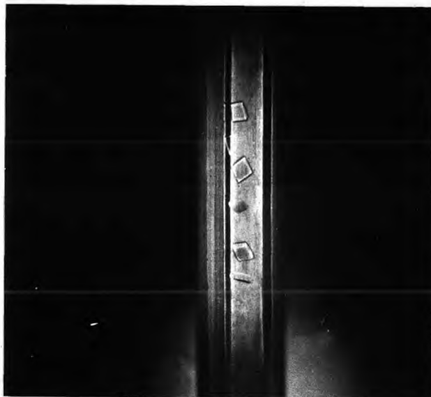
Fig.6.4 Showing irradiated NaCl specimens in the density column.
