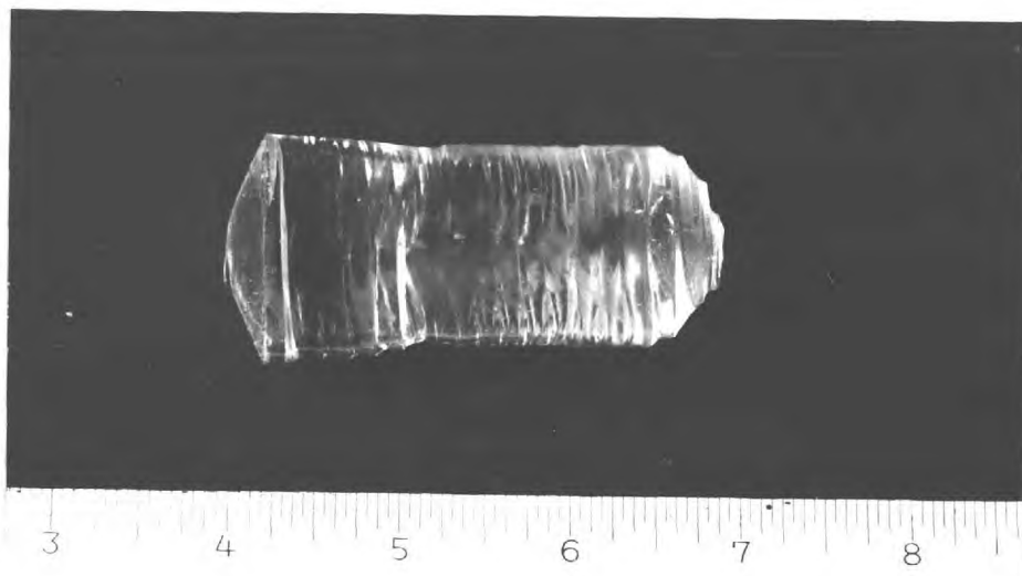
Fig.3.2 Photograph of a typical boule of NaCl single crystal.
