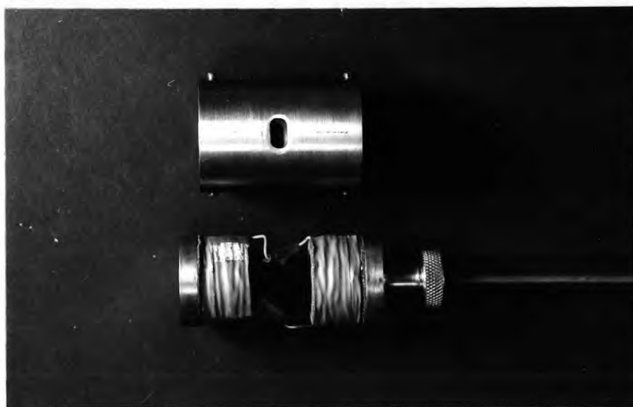
Fig.6.3(b) Exploded view of the deflecting magnet.
