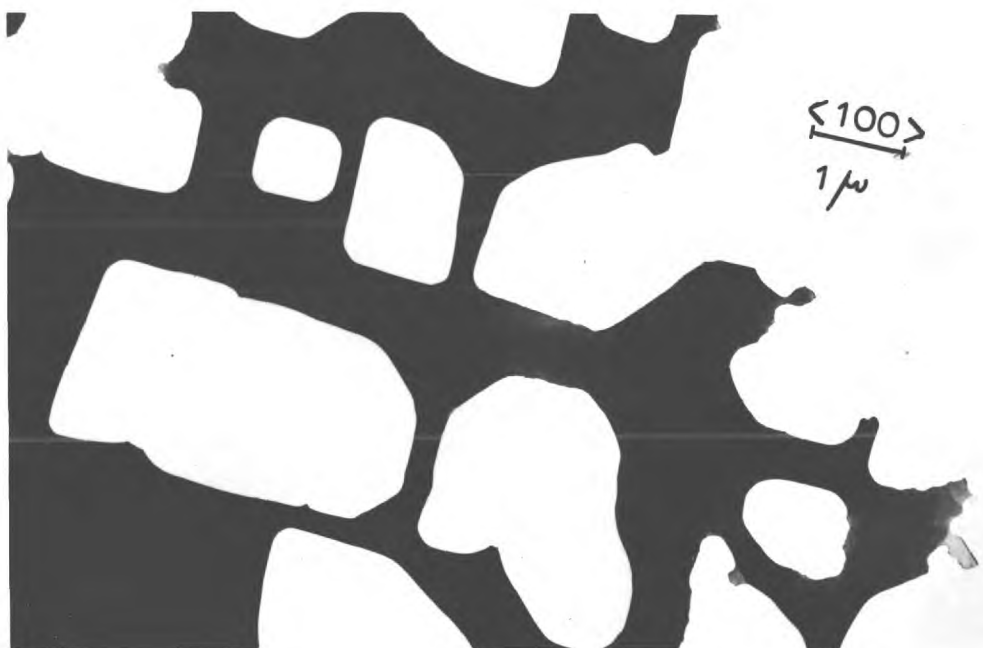
Fig. 4.2. Thinned specimen of \text{CdCl}_2 doped (950 ppm) \text{NaCl} , showing holes in place of the precipitates.
