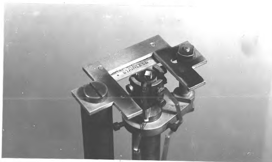
Fig.3.4 Photograph of the cleaving apparatus.
