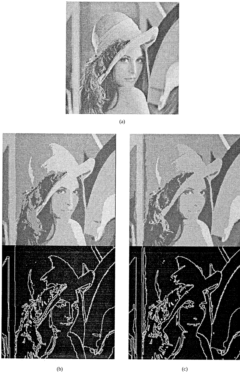
Fig. 5. Segmented images and edge maps of Lenna using the RSST and the FRSST. (a) Original. (b) RSST (350 regions). (c) FRSST (350 regions).
